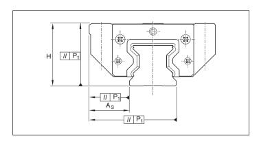
For example, a roller runner block may be used without any problems on various roller guide rails of the same size. Similarly, different roller runner blocks may also be used on one and the same roller guide rail.
