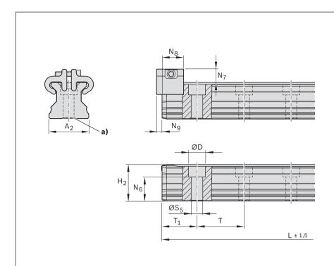
Roller guide rail with cover strip without threaded holes on end faces (not required for strip clamps). Retaining the cover strip with strip clamps (included in the scope of delivery).
