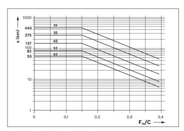
Fig. 3: Relubrication interval
