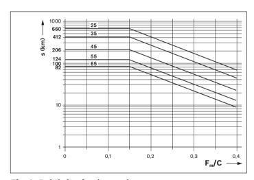
Fig. 2: Relubrication interval
