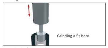
Internal cylindrical grinding
