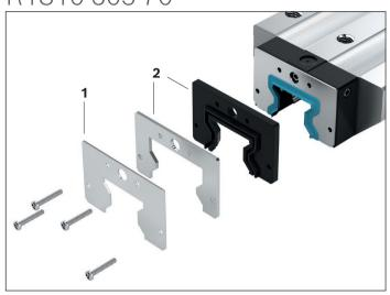
For mounting at the roller runner block FKM seal and cover plate wiper:
