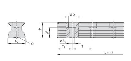
Mounting hole plugs made of plastic are delivered with the roller guide rail and are also available as accessories.
