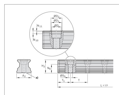
Steel mounting hole plugs are not included in the scope of delivery of the roller guide rails. Order the mounting tool too! For mounting steel mounting hole plugs, see "Mounting instructions for roller rail systems"
