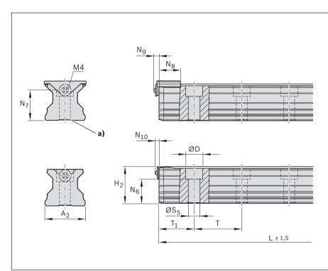
Roller guide rail with cover strip and threaded holes on end faces.
