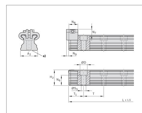
Roller guide rail with cover strip without threaded holes on end faces (not required for strip clamps). Retaining the cover strip with strip clamps (included in the scope of delivery).
