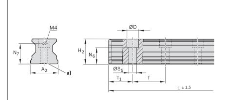
Roller guide rail with front-side thread bore holes without cover strip (cover strip and strip clamp or protective cap are to be ordered separately).
